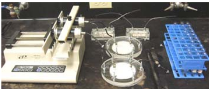
Fig. 5. Experimental setup for testing PDMS-E microreactors.
